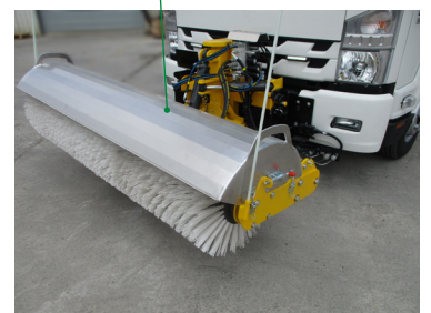
Front Mount Road Broom: Variable sweep pressure on the road surface
