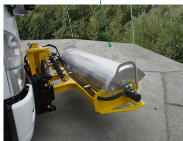
Hydraulic Functions: Angle left and right, tilt left and right, raise and lower
